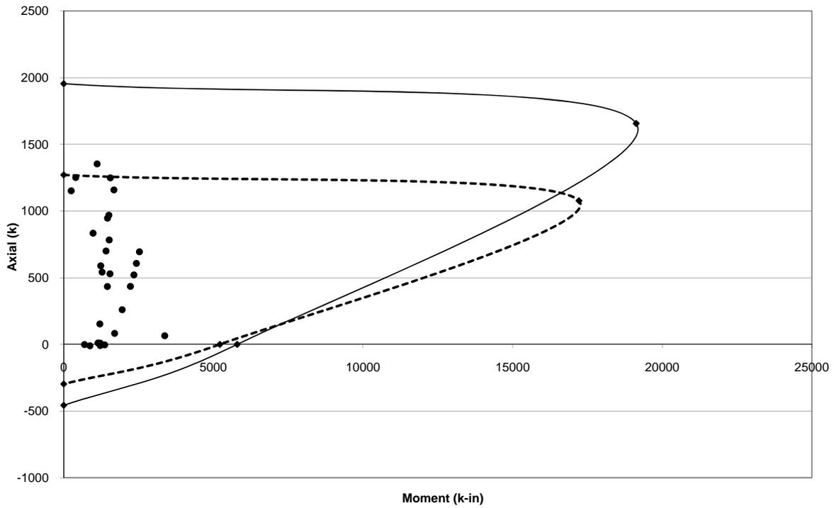
Interaction Diagram for Frame 6 using 1.2D + 1.0L + 0.5Lr + 1.6W
