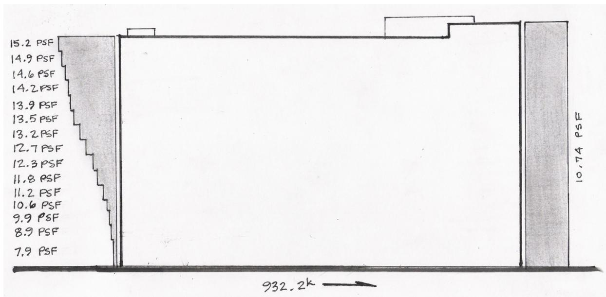
Wind Loading Diagram for East - West Direction:
