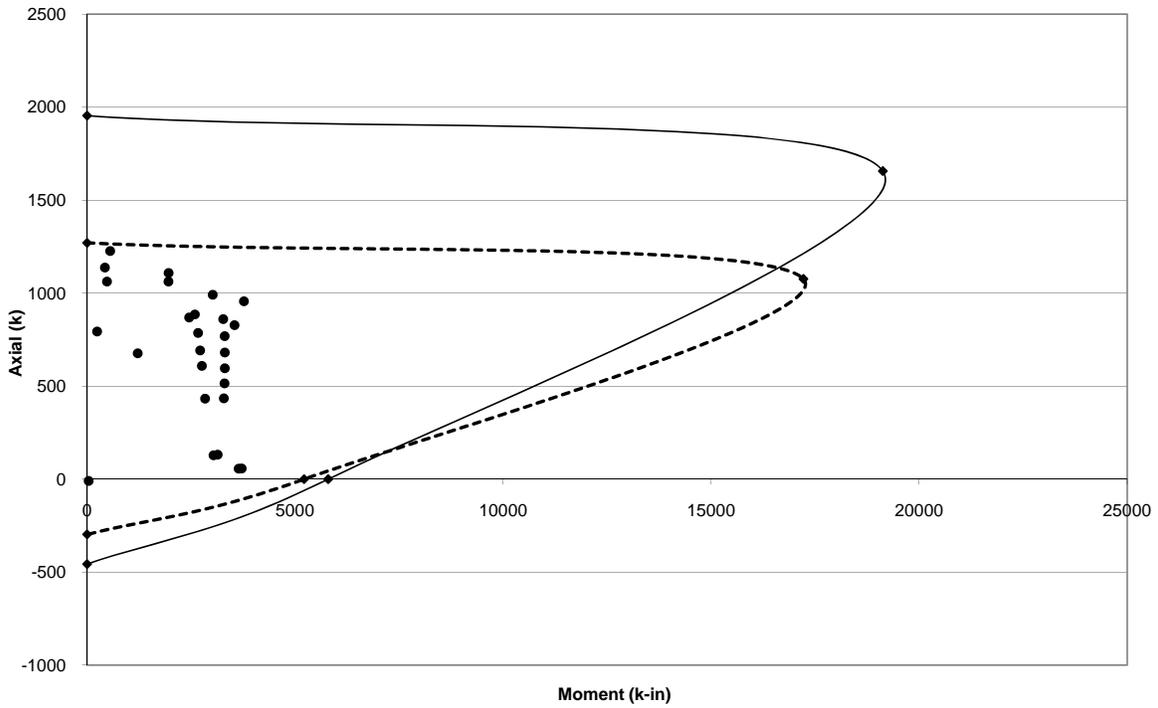
Interaction Diagram for Fram 11 using 1.2D + 1.0L + 0.5Lr + 1.6W
